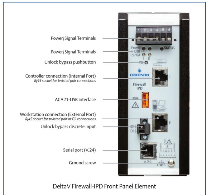
of the DeltaV embedded nodes, the firewall can be deployed in a 1:1 configuration to protect a single node or in conjunction with a DIN-rail mounted network switch to provide a 1:N configuration (a maximum of eight controllers can be connected to the Firewall-IPD). Note that the installation shown in Figure 2 is an example architecture supported for this firewall.
