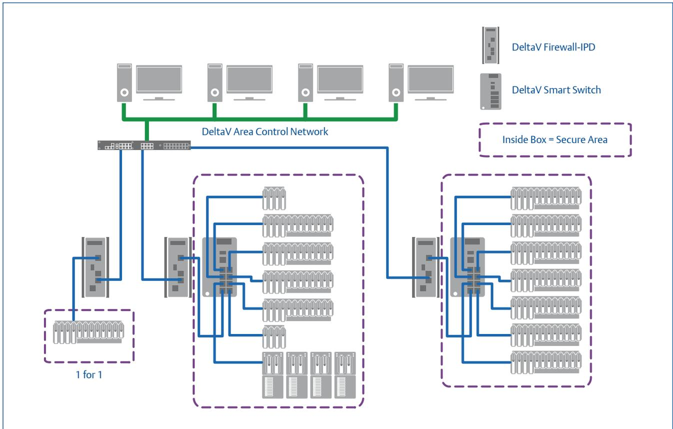
Figure 2 - Typical installation example of the Firewall-IPD in a DeltaV network (Redundant networks not shown for simplicity).
