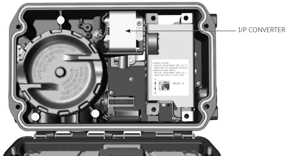
Figure 12. I/P Converter Location
