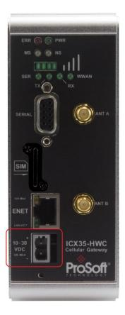
A detachable power connector comes with the radio, as shown below. The connector terminals are labeled + (positive DC connection) and - (DC ground connection).
