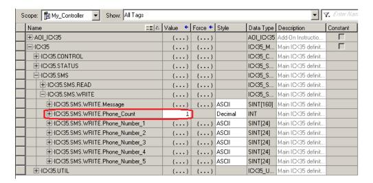
**4** Enter the SMS text message recipient/phone number(s) in the *ICX35.SMS.WRITE.Phone\_Number\_x* controller tag(s).
