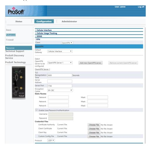
OpenVPN is an open source software application that implements virtual private network (VPN) techniques for creating secure point-to-point or site-to-site connections in routed or bridged configurations and remote access facilities. It uses a custom security protocol that utilizes SSL/TLS for key exchange.
