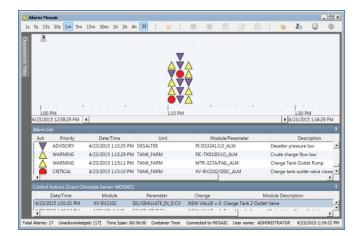
Mosaic relates alarm and control action timing. In this example, the operator can easily check the relevance of the 6 operator actions about 14 minutes before the flood.
