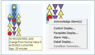
A mouse hover provides easy alarm identification without disturbing current alarm selections. The alarm context menu provides fast display switching, presentation of Alarm Help and Acknowledgement functions.
