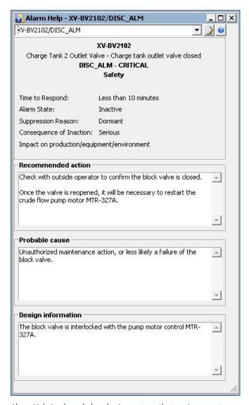
Alarm Help is a knowledge-sharing system, that equips operators to respond quickly and correctly, every time.
