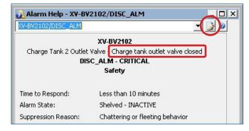
In DeltaV v13, Alarm Help presents alarm descriptions (outlined) and if shelved or out of service, the reason for suppression and current active/inactive state of the alarm.
