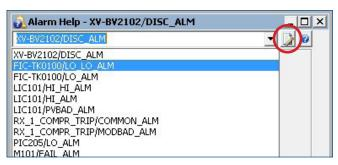
Operators can quickly switch to one of the last ten viewed alarm help entries. Senior operators can add or edit alarm help (circled button ) while in the operator environment.
