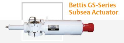
The GS-Series is a scotch-yoke, hydraulic powered actuator especially suited for fail-safe or spring-return operation. The pressure compensated design gives the actuator the capability for shallow or deep water installation.
