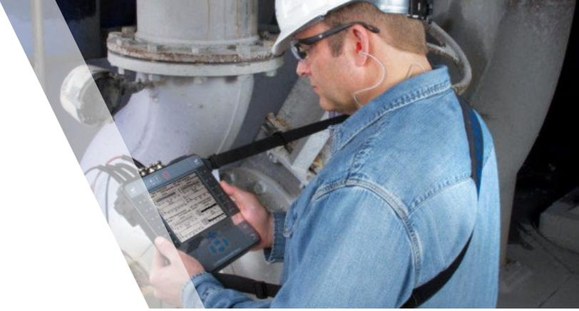
Emerson's PeakVue technology reduces the complexity of machine analysis to provide a simple and reliable indication of equipment health via a single trend.
