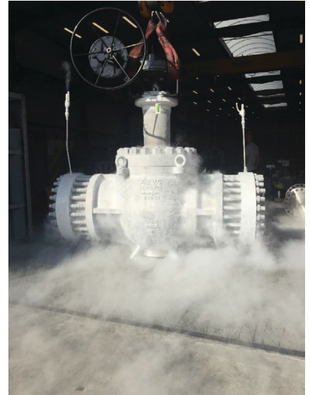
FIGURE 7 AEV 2XC C-Ball Valve after bidirectional cryogenic testing
