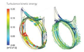
Full round port minimizes any disruption to flow compared to non-round ports, resulting in reduced wear on the valve and downstream components
